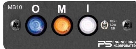
Figure 3, Marker beacon Light Panel
