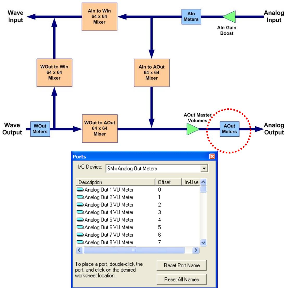
Figure 34, SMx Analog Out Meters Device
