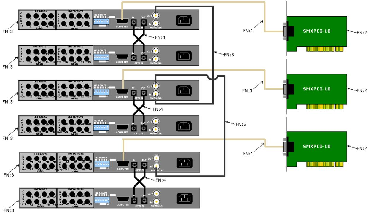
**Figure 22, 48 Channel SMx System Connection Diagram**
