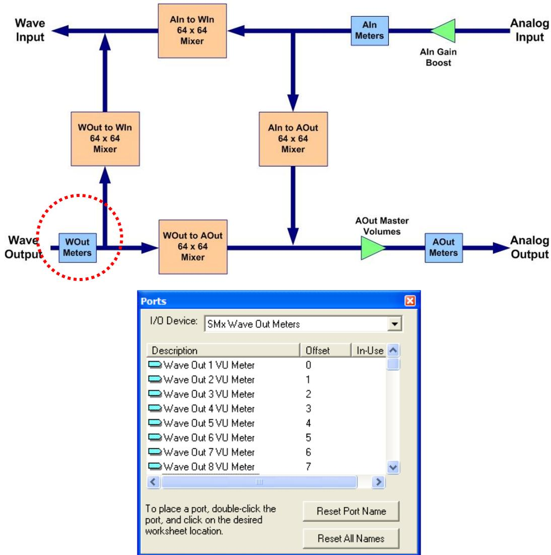
Figure 36, SMx Wave Out Meters Device
