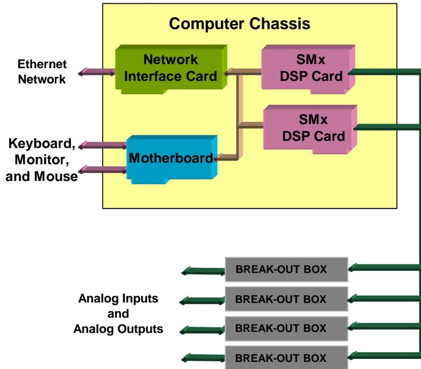
**Figure 2, Overall System Block Diagram**
