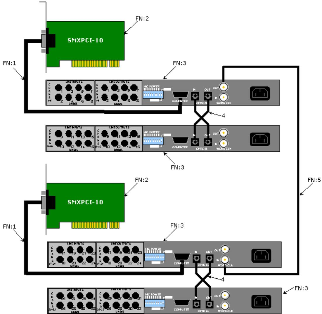
**Figure 20, 32 Channel SMx System Connection Diagram**
