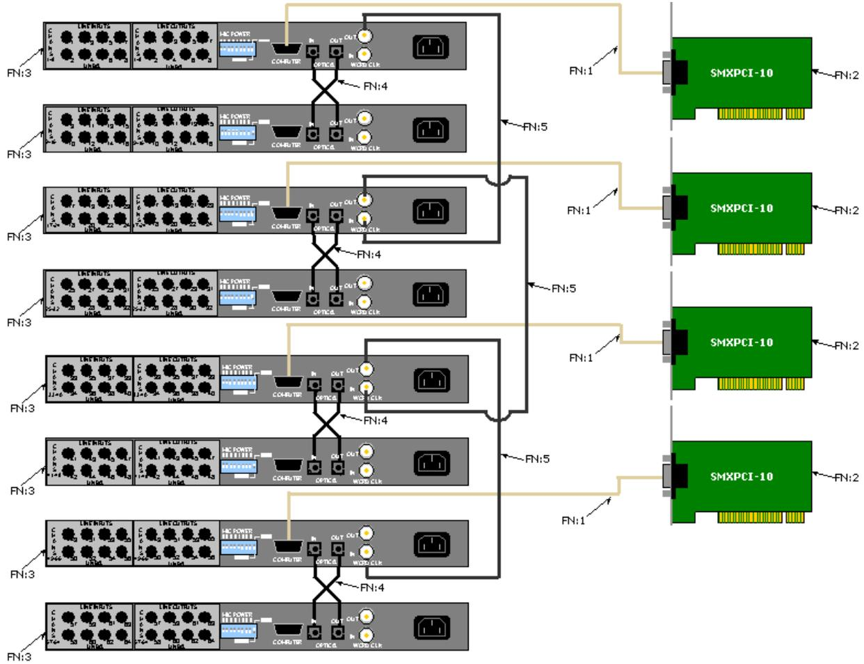
**Figure 24, 64 Channel SMx System Connection Diagram**
