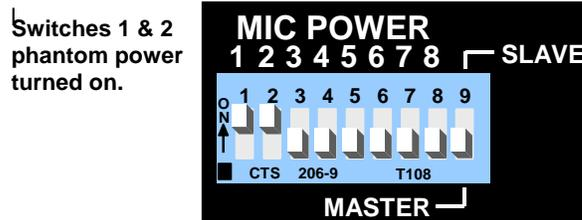
**Figure 15, Breakout Box Phantom Power Switches**
