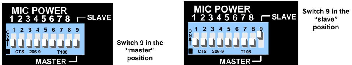
**Figure 14, Breakout Box Master/Slave Dip Switch**
