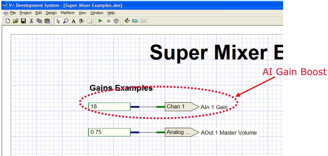
Figure 41, AI Gain Boost Example
