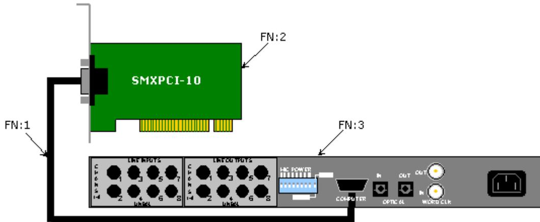
**Figure 17, 8 Channel SMx System Connection Diagram**
