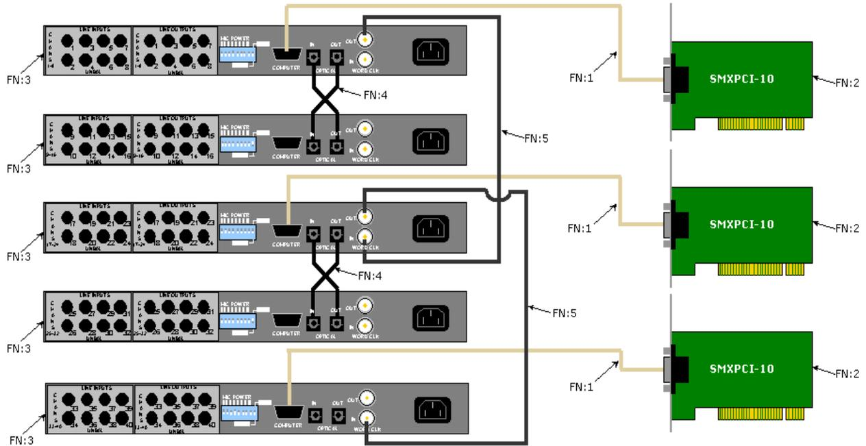
**Figure 21, 40 Channel SMx System Connection Diagram**
