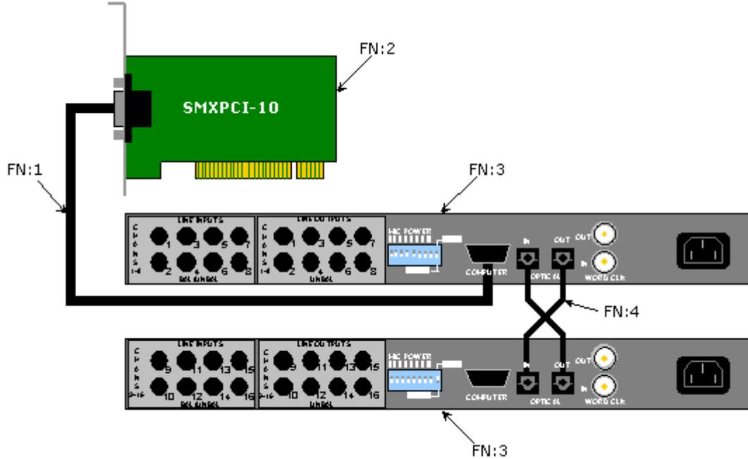
**Figure 18, 16 Channel SMx System Connection Diagram**
