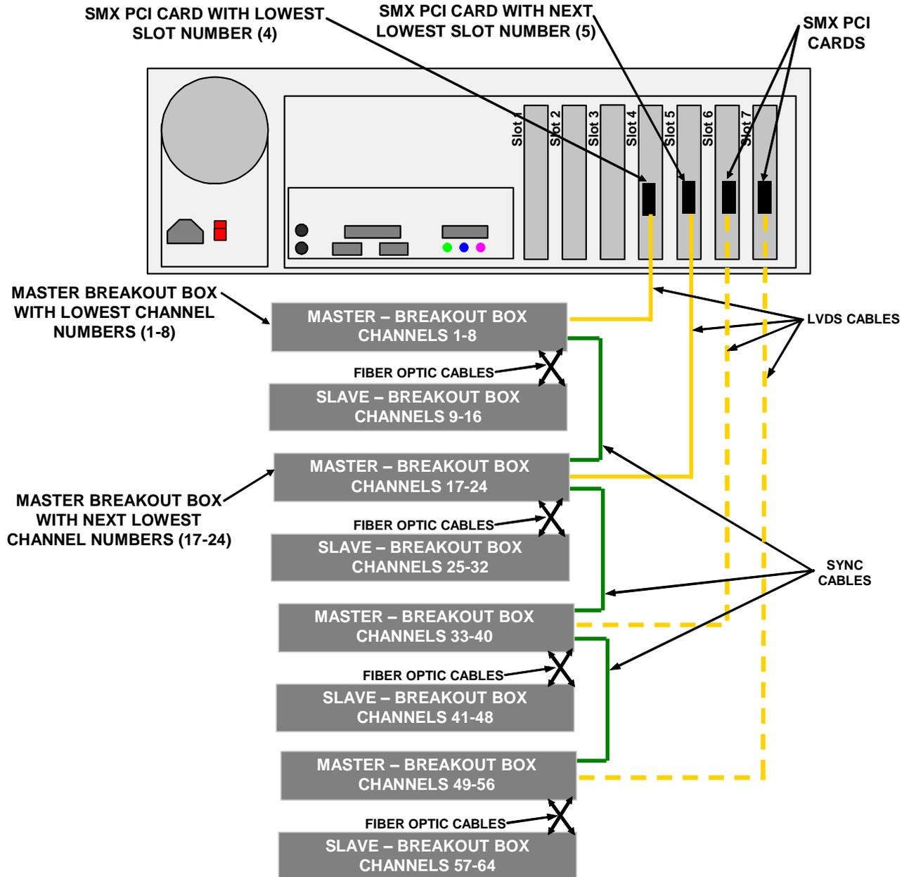
**Note:** The SMx PCI card with the lowest slot number (4) is connected to the Master – Breakout Box with the lowest channel numbers (1-8). The SMx PCI card with the next lowest slot number (5) is connected to the Master – Breakout box with the next lowest channel numbers (17-24). etc.
