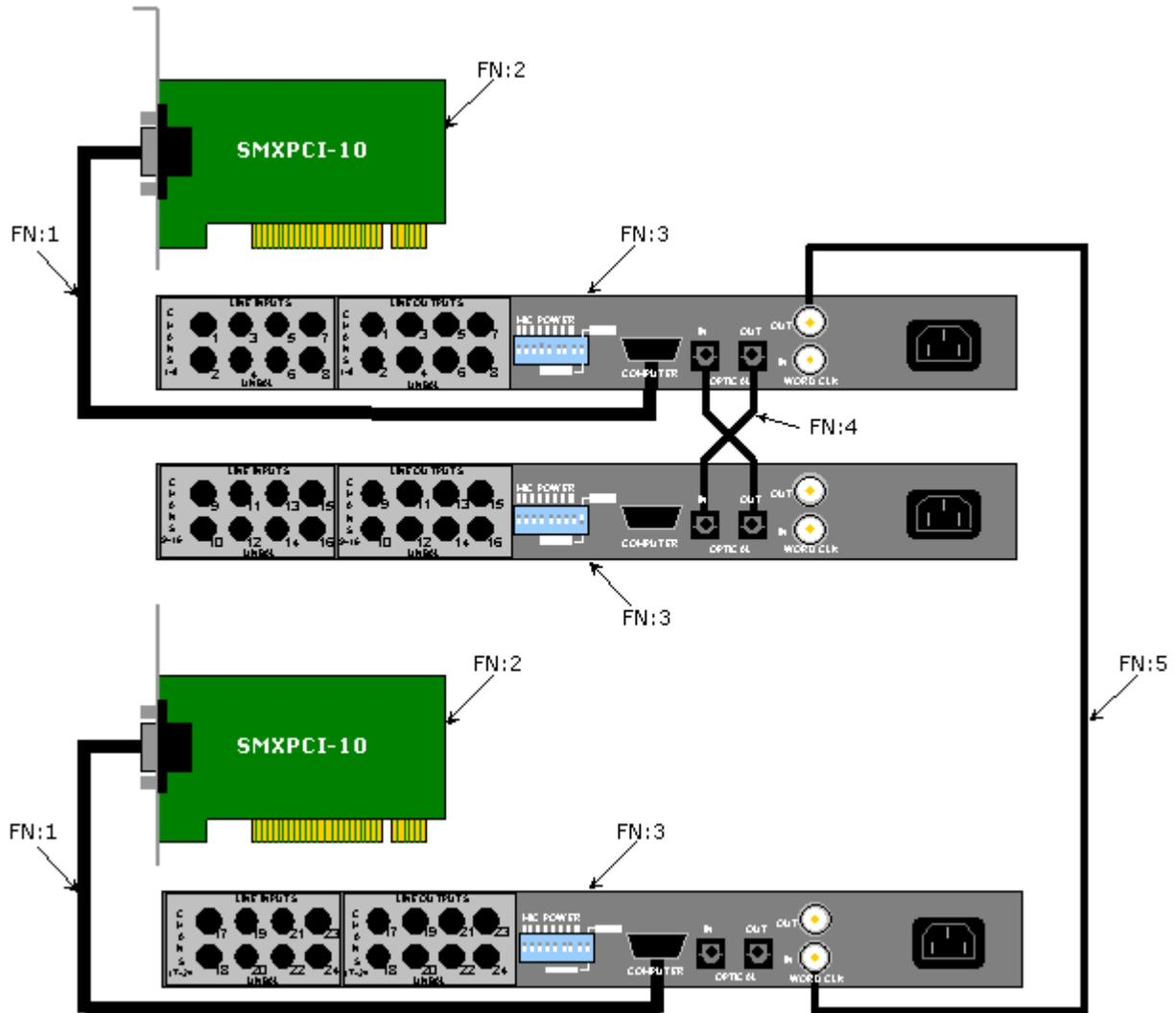
**Figure 19, 24 Channel SMx System Connection Diagram**
