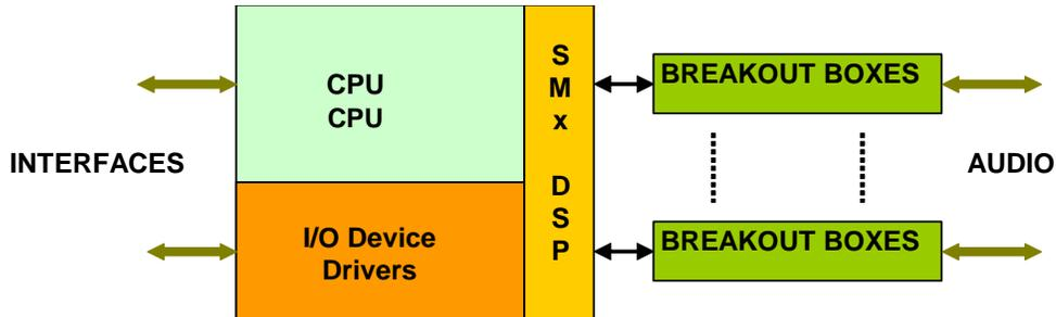
**Figure 1, SMx System Architecture**
