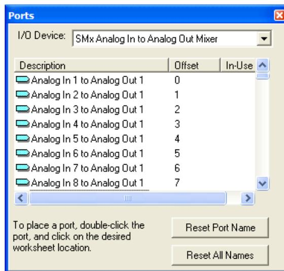
Figure 31, SMx Analog In to Analog Out Mixer Device
