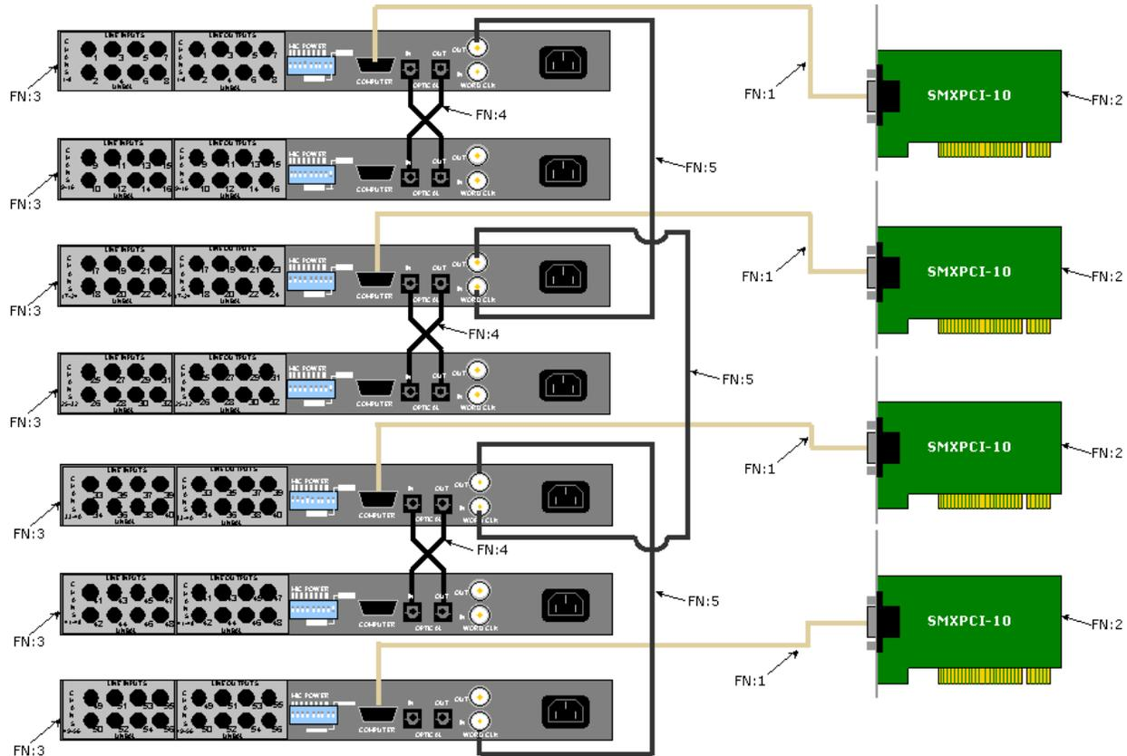
**Figure 23, 56 Channel SMx System Connection Diagram**
