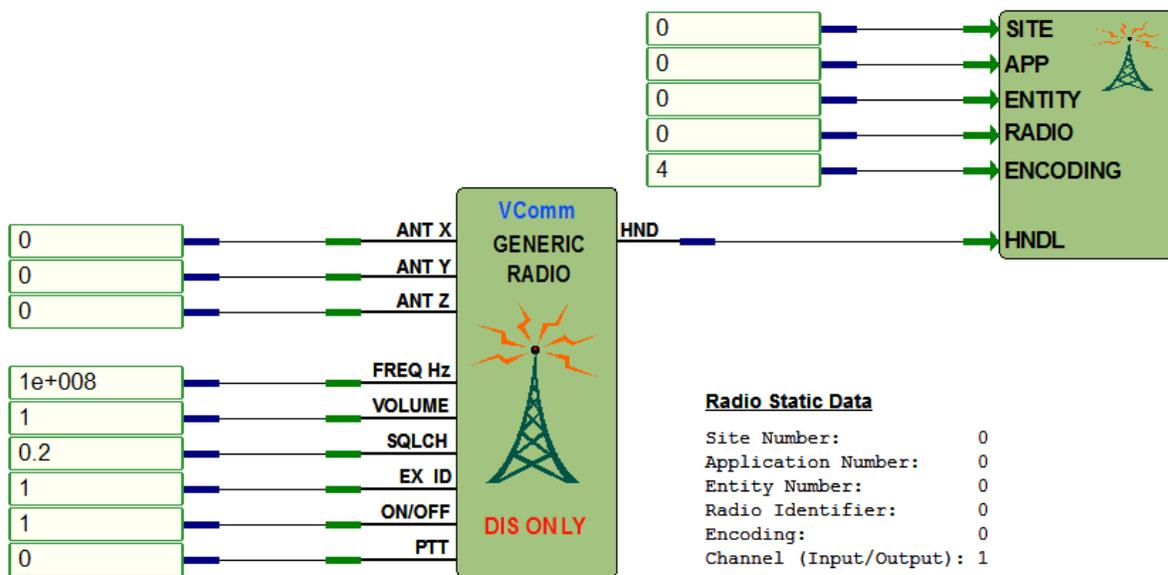
Figure 41, Setting DIS Radio Identifiers Dynamically
