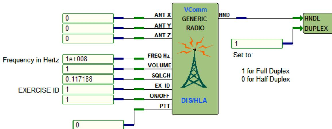
Figure 69, Object 2041 - VComm Set Radio Duplex Mode
