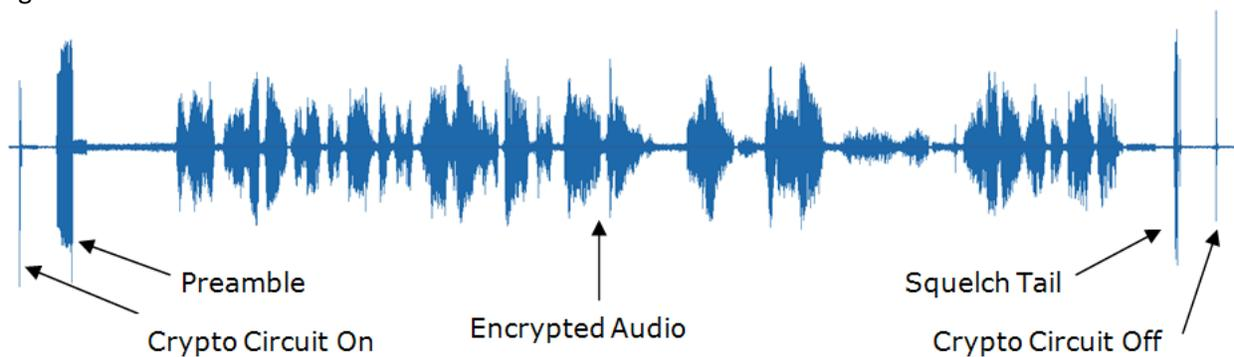
Figure 63, Example KY-58 Reception of Secure Transmission
