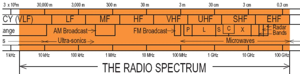
**Figure 13, the Radio Frequency Spectrum**
