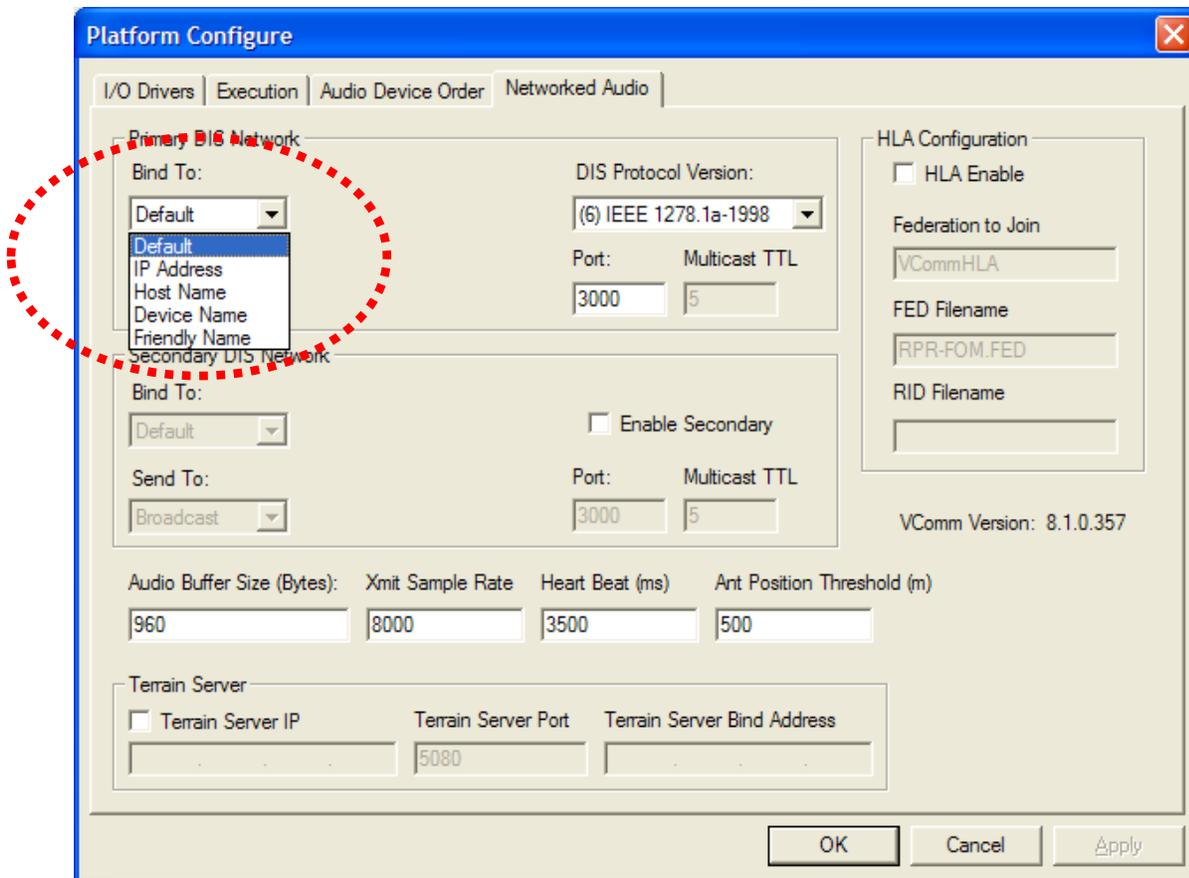
**Figure 10, Networked Audio Binding Dropdown**
