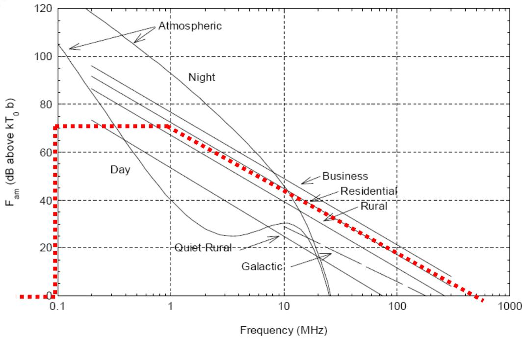
Figure 32, VComm Atmospheric Noise Model
