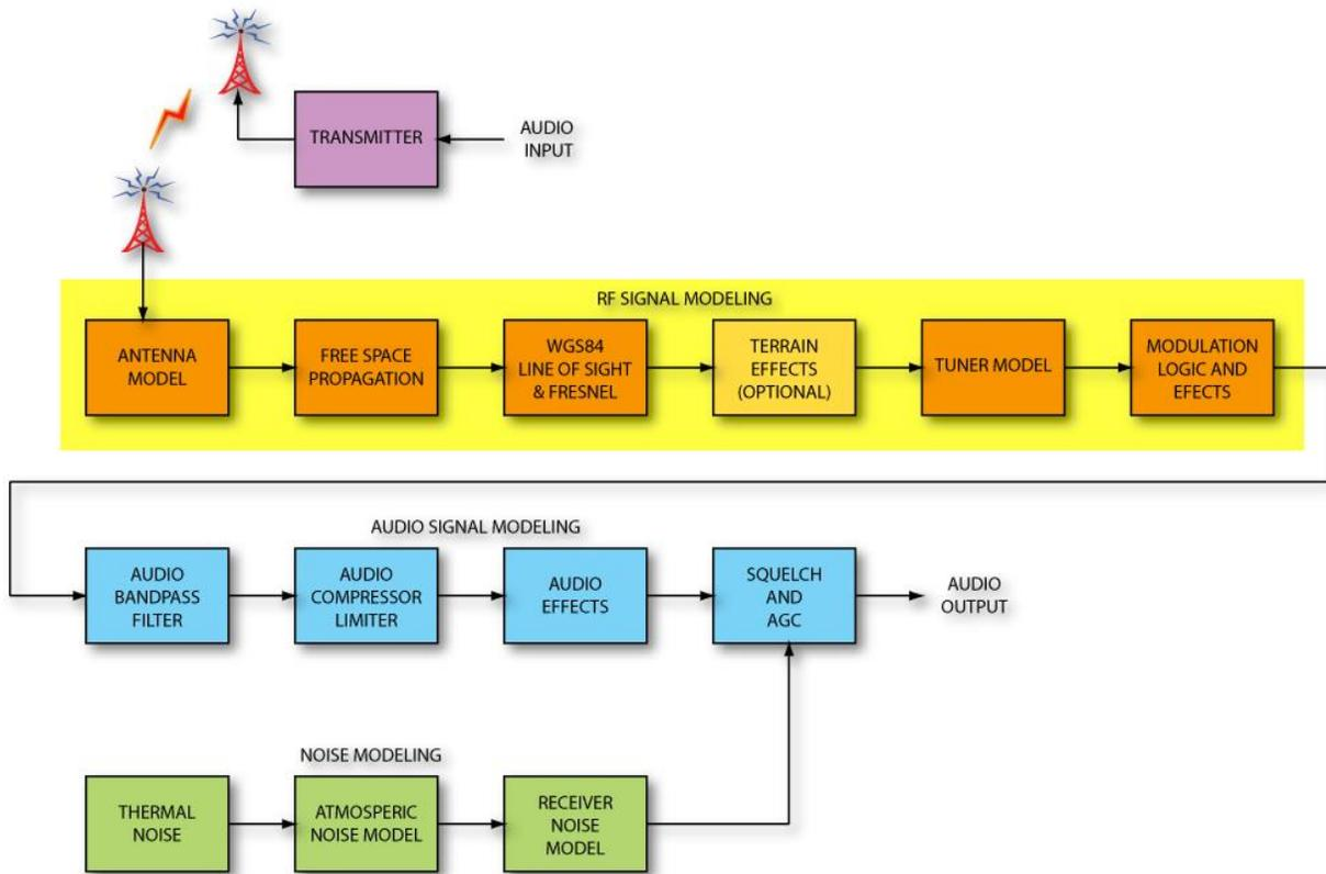
Figure 15, VComm RF Signal Modeling
