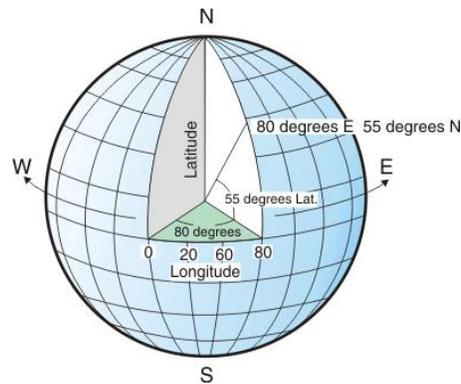
Figure 46, Geodetic Coordinate System
