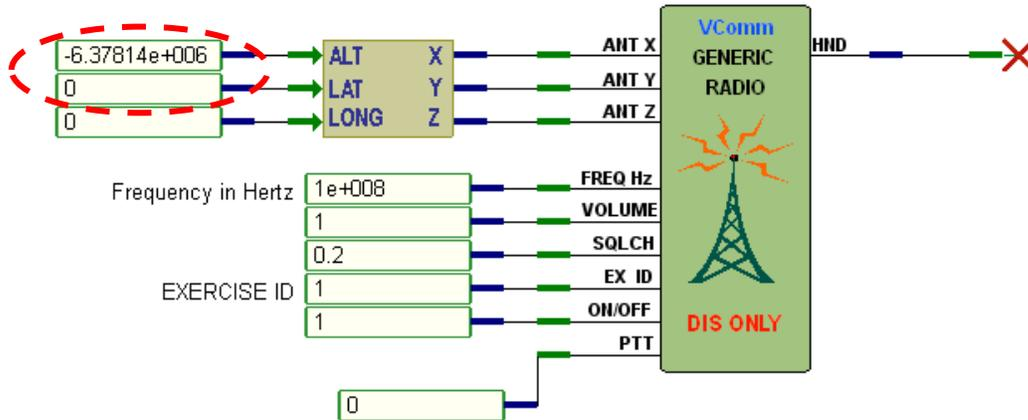
**Figure 49, Setting Position to Geocentric (0,0,0)**
