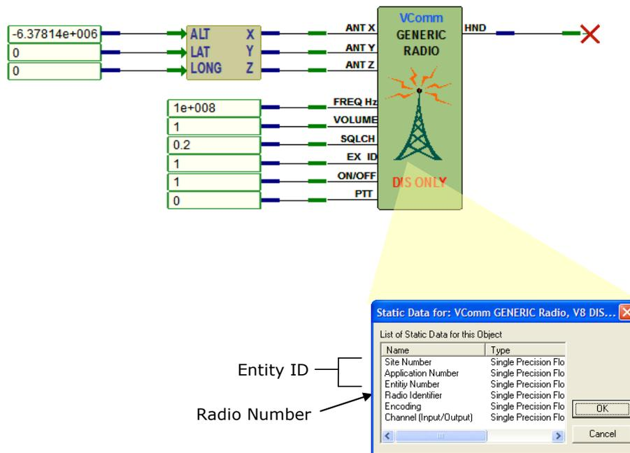
**Figure 40, Setting DIS Radio Identifiers via Static Data**
