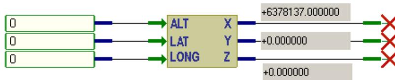
Figure 48, Object 2029 – ALT, LAT, LONG to Geocentric Conversion
