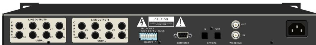
**Figure 5, SimPhonics SMx Breakout Box**
