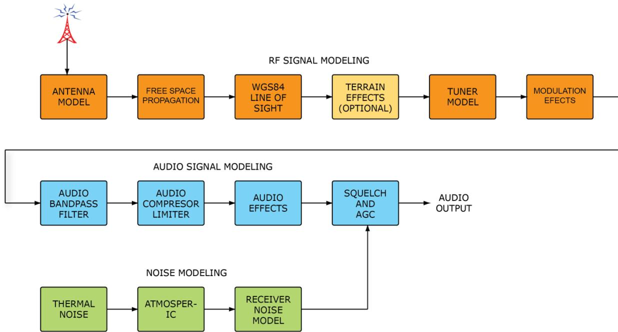
Figure 14, VComm Radio Modeling Functional Flow
