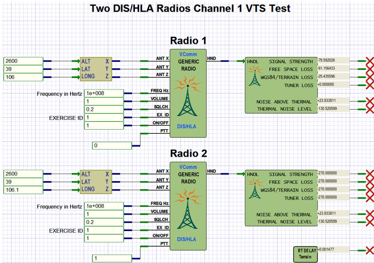
Figure 20, Example Design Using the VComm Terrain Server
