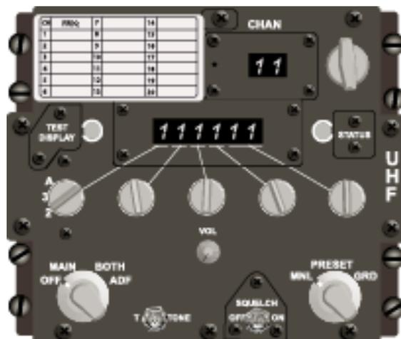
**Figure 53, AN/ARC-164 Radio Control Head**
