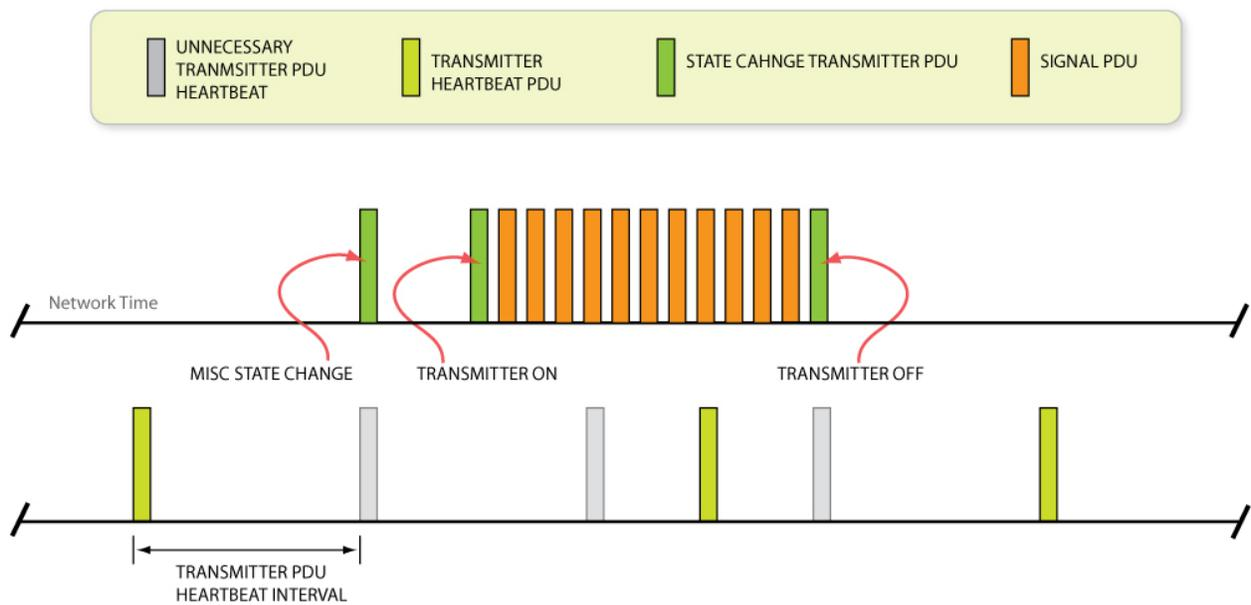
Figure 34, Transmitter and Signal PDU Time Sequencing
