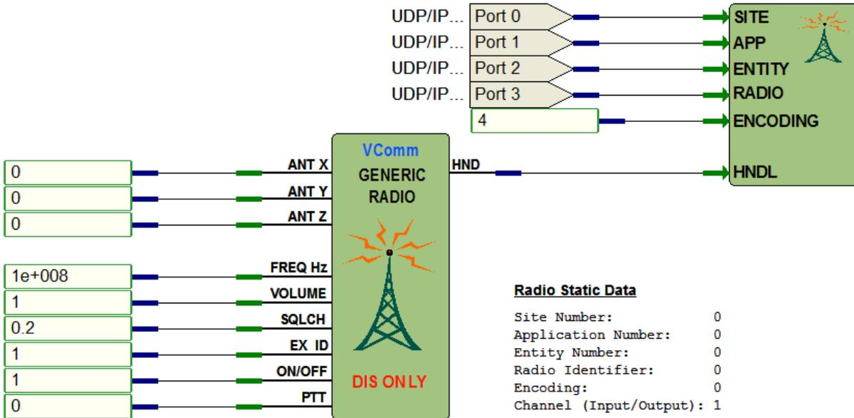
**Figure 42, Using an External Interface to set a Radio Identifier**
