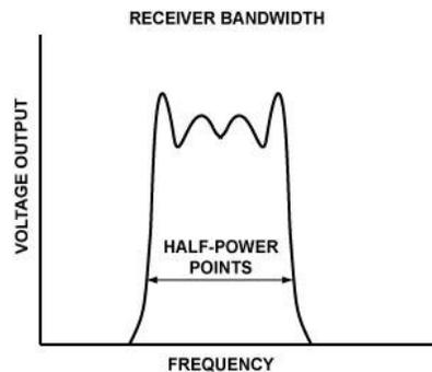
**Figure 25, VComm Tuning Response Curve**
