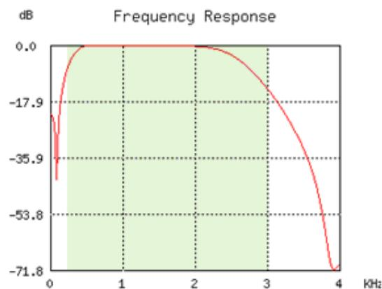
**Figure 29, Object 2055 Frequency Response at an 8K Sampling Rate**
