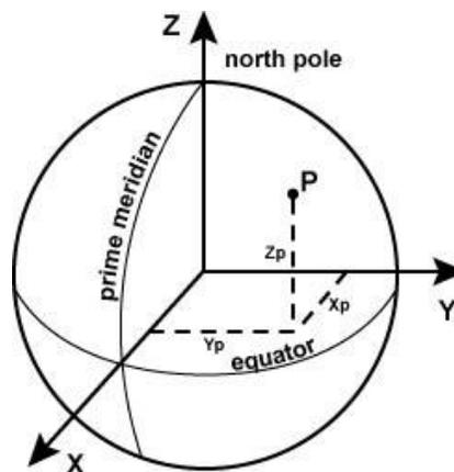
Figure 47, Geocentric Coordinate System
