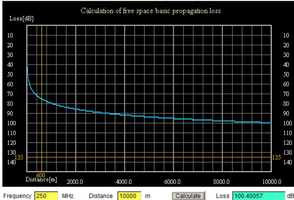
**Figure 17, Free Space Propagation Loss**
