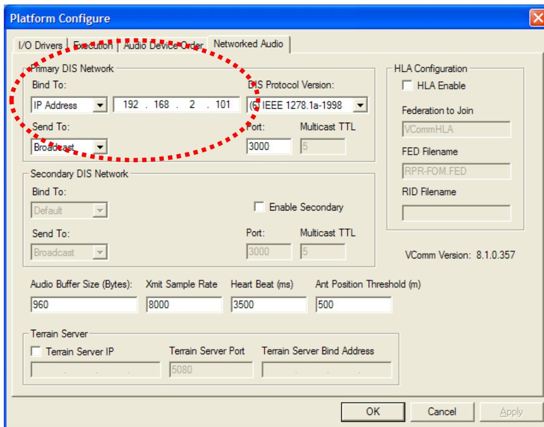
**Figure 11, Networked Audio Binding To IP Address**
