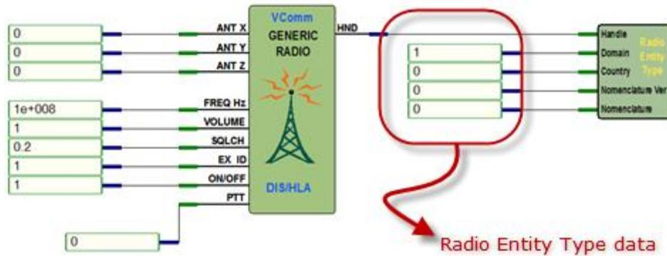
**Figure 38, VComm Radio Entity Type Object**
