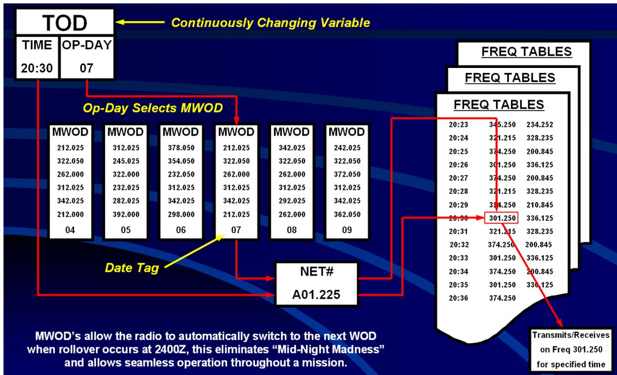
Figure 55, HAVE QUICK Operational Diagram Example
